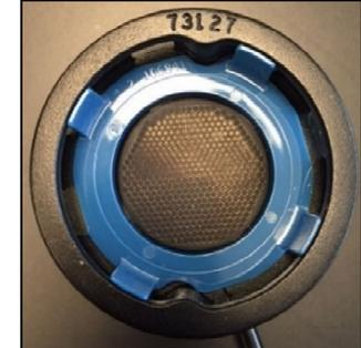
Figure 17: Ultrasonic Sensor with Mesh
