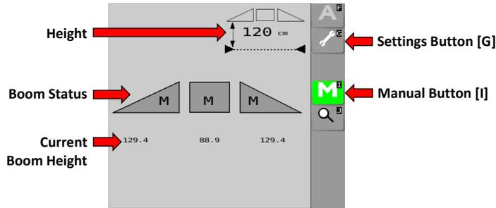
Figure 1: NORAC UC7 Run Screen – Manual Mode
