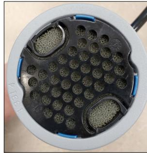
Figure 16: Ultrasonic Sensor with Retainer Clip
