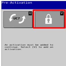
Power on the display terminal. The first screen should prompt for an activation code. Press the lock button (V).
