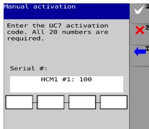
Enter the activation code provided for the specific make/model of sprayer. Select the check button (F).
