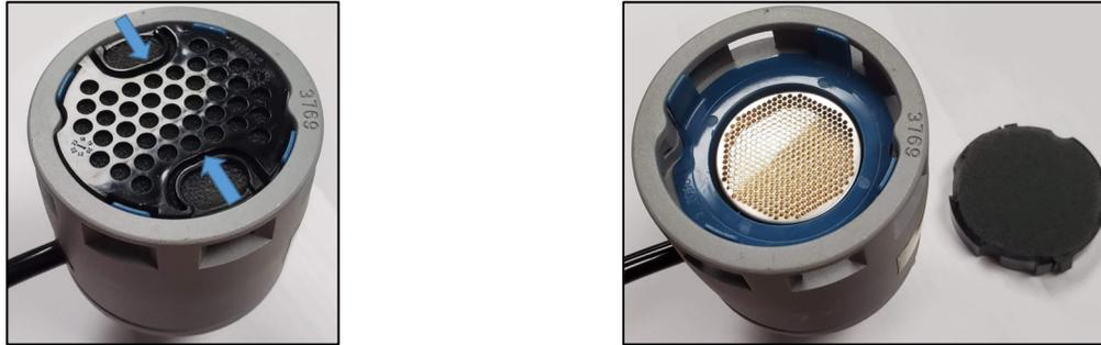
Figure 18: Sensor Foam Retainer Clip Removal
