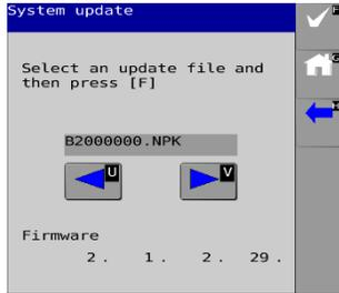
Select the update file to use. Press the [F] button. Wait while the system updates. Turn the machine off and on when the update is complete. If the sensors need to be updated, the system will take longer than normal to load onto the display. Complete one additional power cycle after the system loads onto the display. An automatic setup will need to be performed each time a firmware update is completed.
