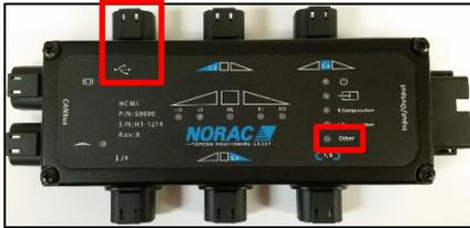
Insert a USB drive loaded with the XXXXXX.npk update file into the USB connector on the HCM1. The LED marked Other will be solid green when the USB is recognized.
