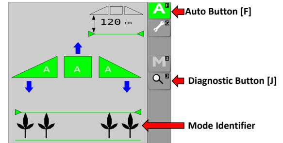
Figure 2: NORAC UC7 Run Screen – Automatic Mode
